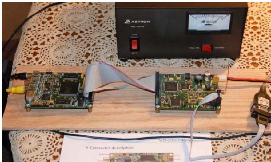
Figure 2 – MPEG2 and DVB-S 1.2 GHz Exciter from SR-Systems on the Test “Breadboard”
