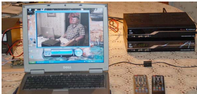
Figure 22 – Bench testing the ViewSat STB that will be used at Orange PD
