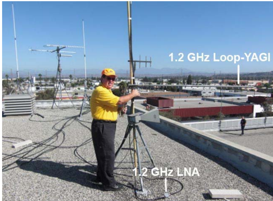
Figure 12 – Robbie KB6CJZ adjusts the Receiver’s 1.2 GHz Loop-Yagi antenna
