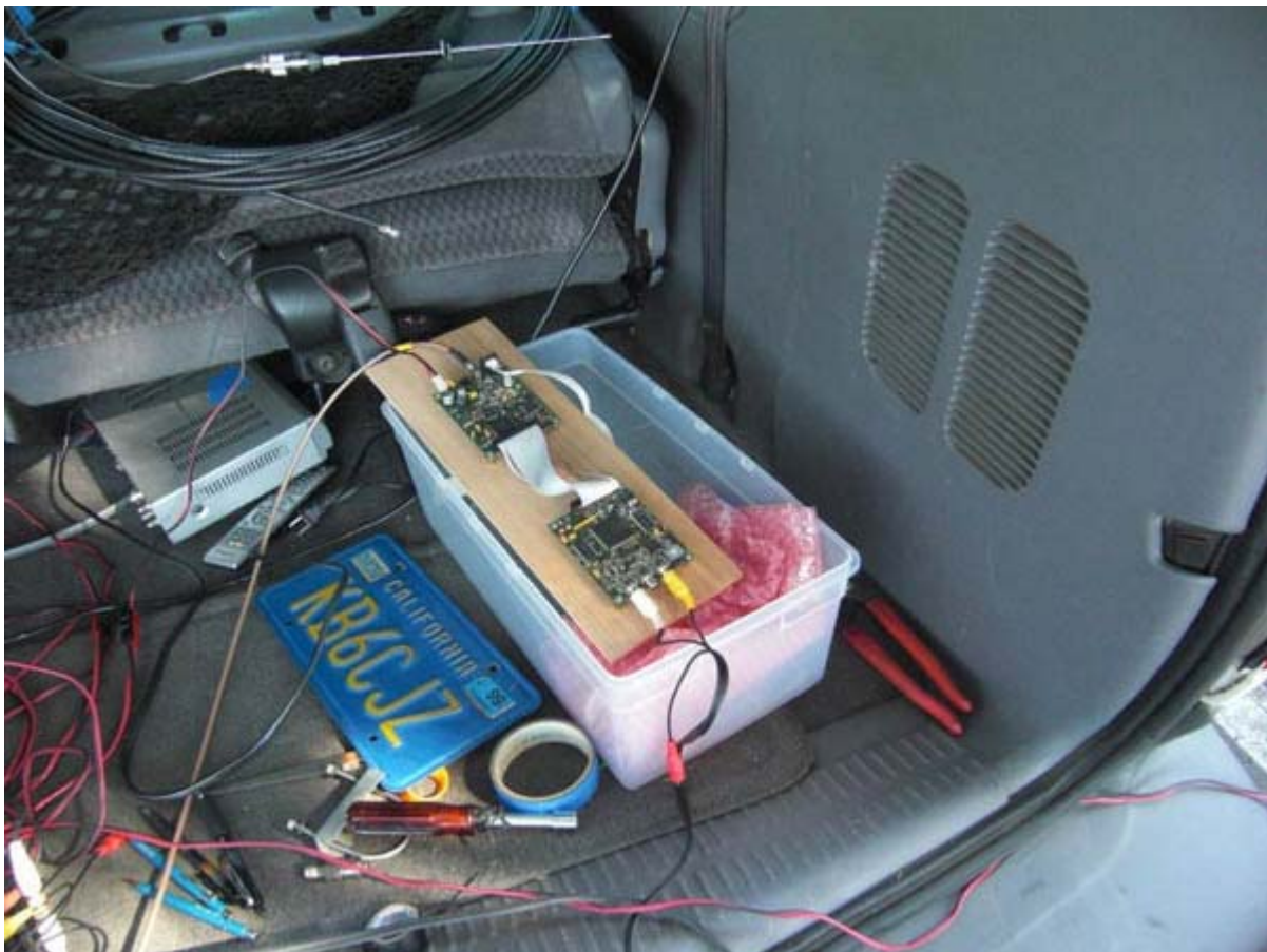
Figure 11 – DATV DVB-S 1 mW Transmitter for 1.2 GHz
