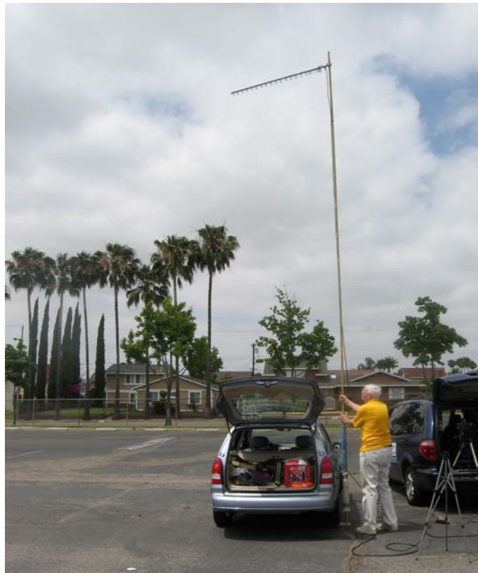
Figure 24 – Bruce KC6DLA adjusts direction for the Field set-up of the 1.2 GHz Transmitting Loop-Yagi Antenna
