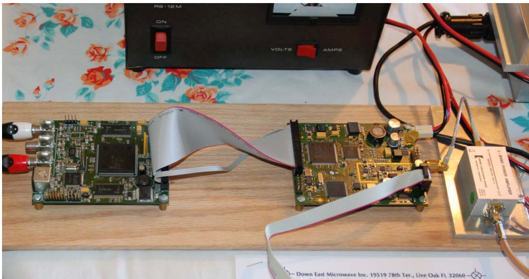
Figure 16 – Breadboard of MPEG-2 Board and MiniMod Exciter Board and the Kuhne 1st-Stage PA (on right side)
