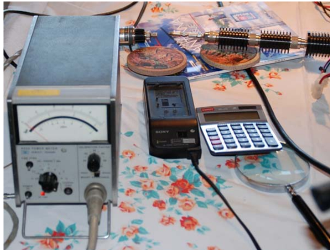
Figure 19 – HP Model 432A Power Meter Note the attenuator-stack at the top of the photo
