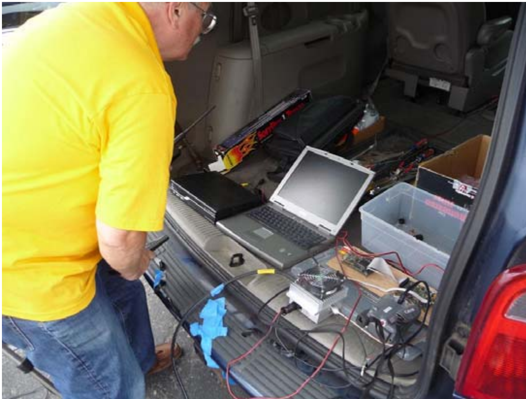
Figure 25 – Field DATV transmitting station in back of MiniVan (the “sniffer receiver” display is seen in center)
