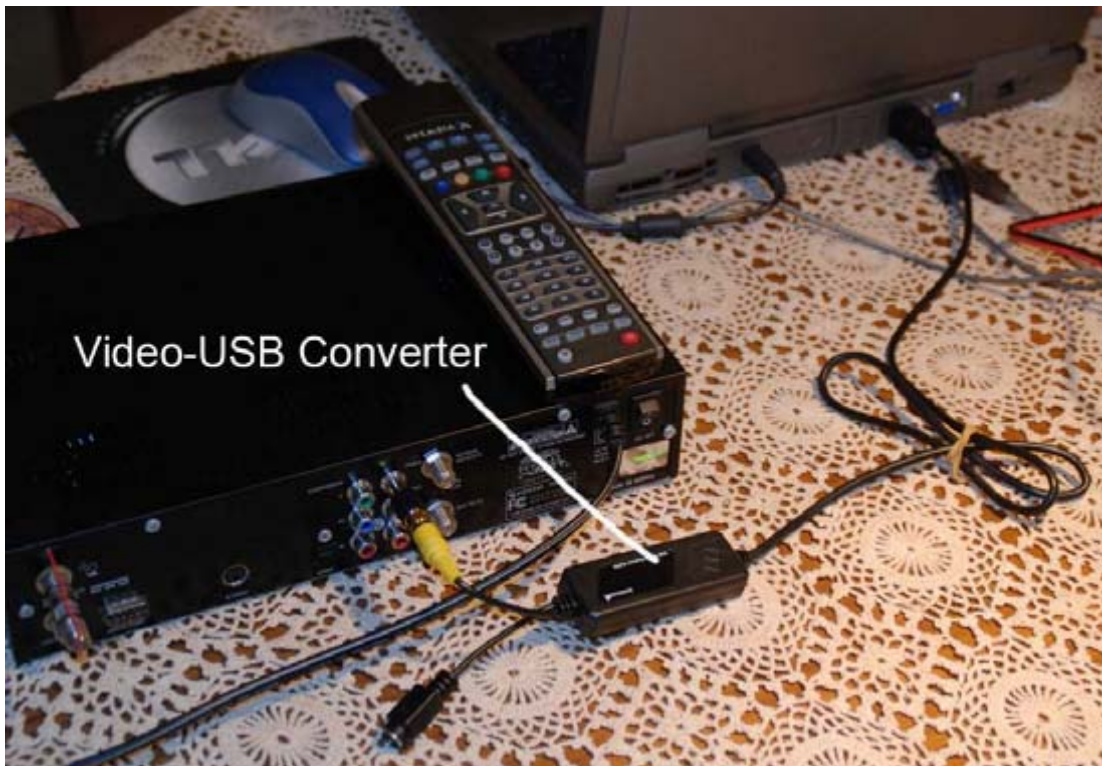
Figure 4 – The Composite-Video-to-USB converter sends the STB Video to the Computer USB Port
