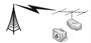
Fig 1 Terrestrial reception using commercial set-top box
