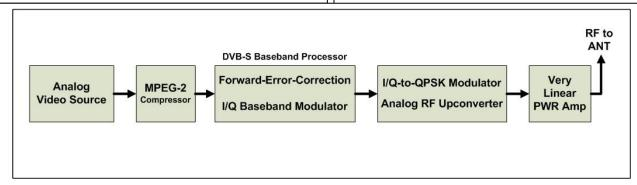
Figure 2 – Block Diagram of DVB-S Transmitter for Digital-ATV
