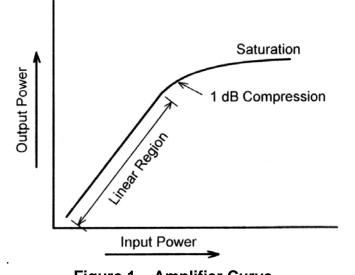
Figure 1 – Amplifier Curve
