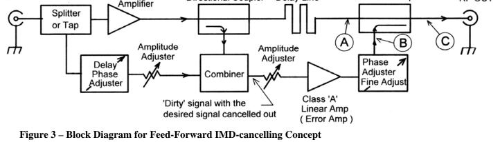
The signal with high levels of IMD at (A) is combined with the out of phase "dirty" IMD signal from (B) which cancels the IMD, to produce a desired clean signal with 20 to 30 dB lower IMD at (C)
