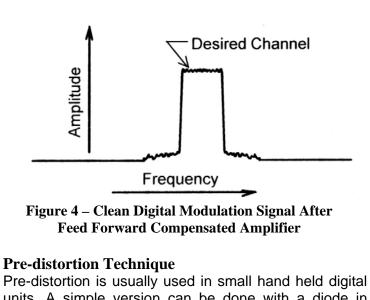
units. A simple version can be done with a diode in series with the RF path prior to the driver amplifier and is slightly biased and its parameters chosen to compliment the drive levels used [see **Fig 5**]. The bias current is adjustable to allow optimizing the predistortion; this method can give about a 6 dB improvement in lowering IMD.
