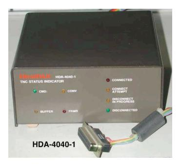
Heathkit offered the HD-4040-1 Status Indicator which decodes information on the parallel port of the HD-4040 (or any TNC-1's parallel port) and provides status in the form of eight LED lamps. It also provides an audio tone to signal when someone connects - this turned out to be a very good feature as it is hard to no-
