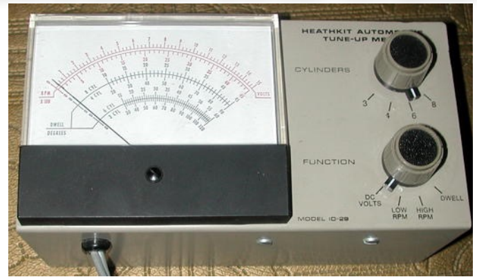
Figure 1: Heathkit ID-29 Automobile Tune-up Meter (Shown less plastic case).
