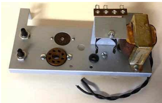
Figure 6: The V-6 chassis, cleaned, coated and partially populated with parts.
