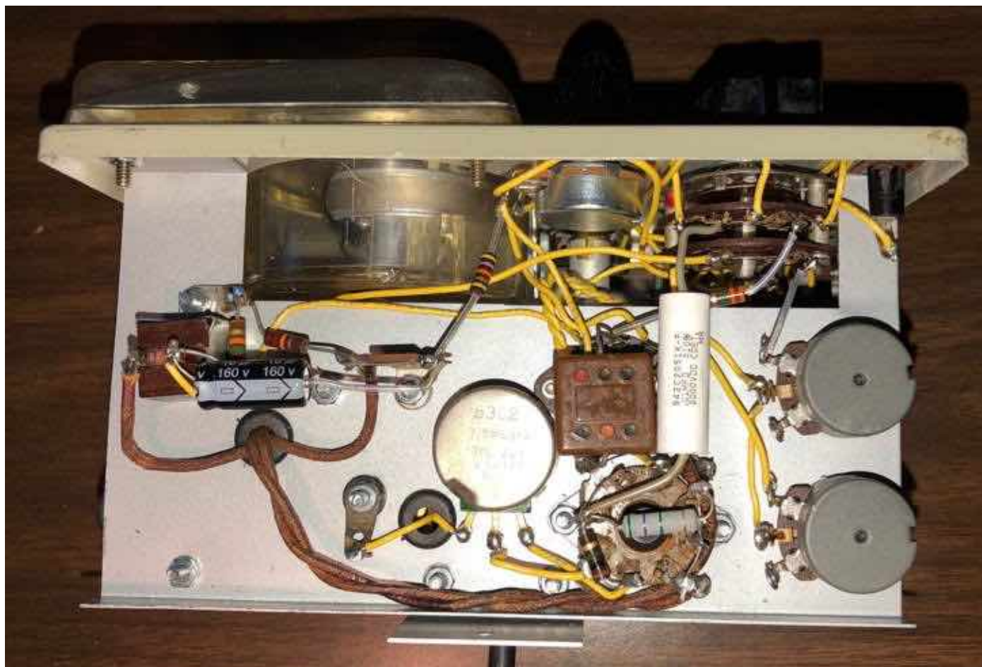
Figure 13: Chassis left side, showing "siliconized" selenium rectifier (left), 7.5 M Ω potentiometer (lower center), old style mica capacitor and new 0.01 2,000V capacitor (above octal tube socket), and function switch (in cutout, to right).
