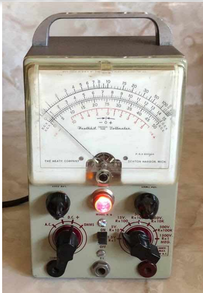
Figure 1: Completed restoration of the Heathkit V-6 VTVM during burn-in. The slight meter offset is intentional and indicates the circuit continues to function.
