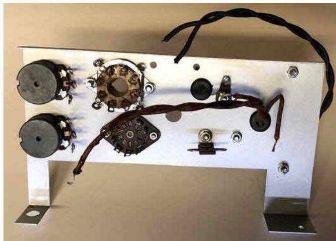
Figure 9: The underside of the chassis prior to wiring. The adjustment pots and tube sockets are original but cleaned and tested. The vacant hole is for the 7.5 MΩ pot.
