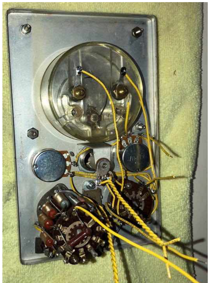
Figure 10: The underside of the chassis prior to wiring. The adjustment pots and tube sockets are original but cleaned and tested. The vacant hole is for the 7.5 MΩ pot.
