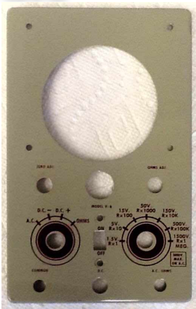
Figure 7: The front panel cleaned up nicely with just some Dawn detergent and warm water.
