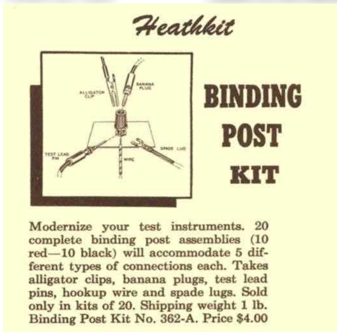
Figure 11: Heath was so proud of their new 5-way binding post they offered them separately in packs of 10 pairs for many years (1953-54 Winter Flyer Ad).
