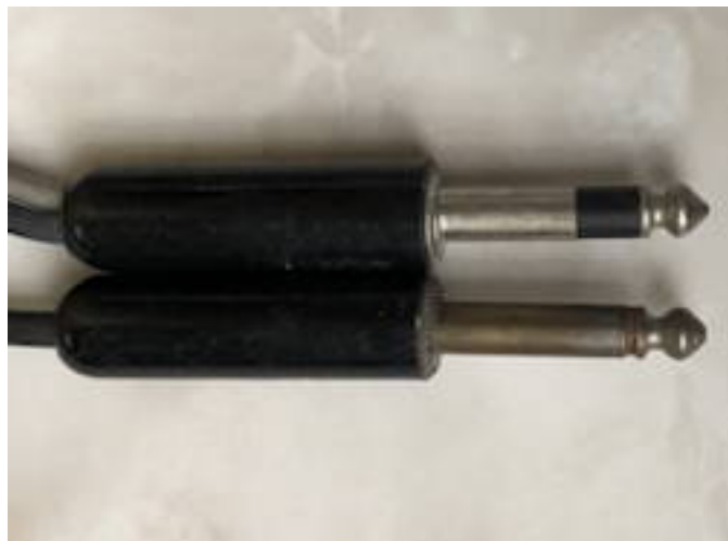
Figure 7: Top shows the new phone plug with its thicker insulation to prevent flashover at higher voltages. Below it is the standard phone plug used on the earlier VTVMs.
