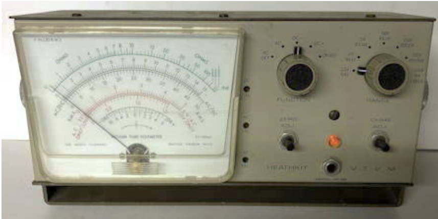
Figure 8: Heathkit IM-28 Deluxe "Service Bench" VTVM In the "New Look" style. It is the first of the series to use a 120/240 V primary transformer and a three-wire AC plug. Photo by author.
