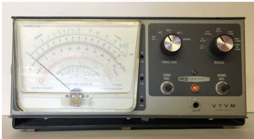
Figure 6: Heathkit IM-13 Deluxe "Service Bench" VTVM In the Classic II style, and in the new horizontal format. Note calibration access holes to the right of the meter. Photo by author.
