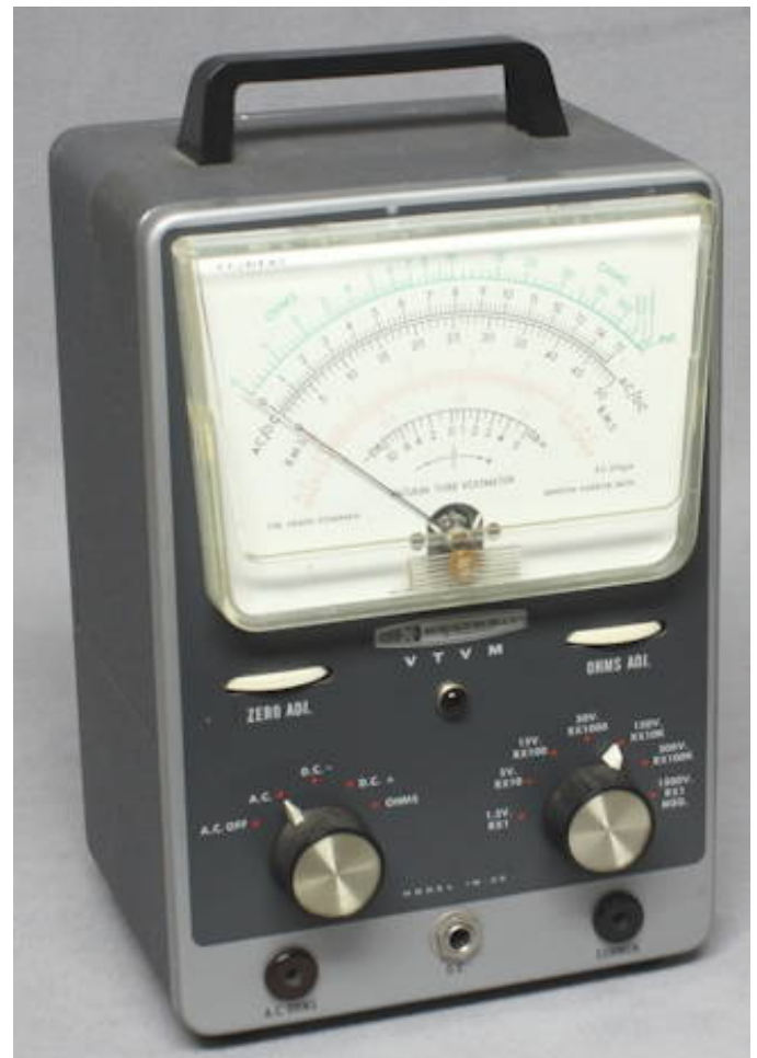
Figure 5: Heathkit IM-32 Deluxe "Service Bench" VTVM The Classic II style update of the IM-10. It was the last of the vertically oriented Bench VTVM. Photo courtesy of Sonny Clutter, www.radiolaquy.com .
