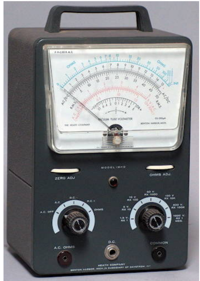
Figure 1: Heathkit IM-10 "Deluxe Service Bench" VTVM. The first of the Service Bench VTVM series, vertically configured with the controls below the large 6" meter. Photo courtesy of Chuck Penson - WA7ZZE.
