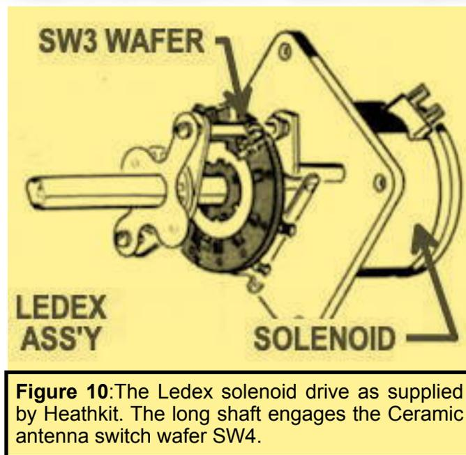
**Figure 10:**The Ledex solenoid drive as supplied by Heathkit. The long shaft engages the Ceramic antenna switch wafer SW4.
