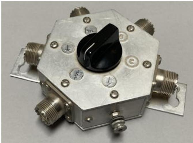
**Figure 2:** The HD-1234 Manual Antenna Switch with its five female UHF connectors and a ground post. Photo by Chuck Penson - WA7ZZE
