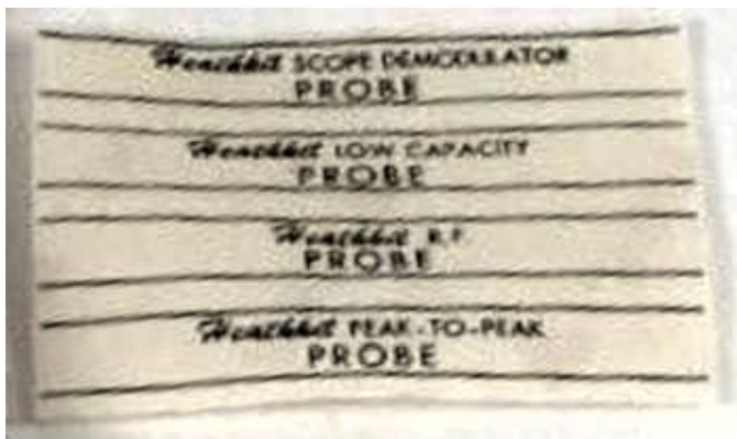
Figure 12: The decal sheet, (Part # 390-13) provided with later probes using the red - aluminum - black probe body.
