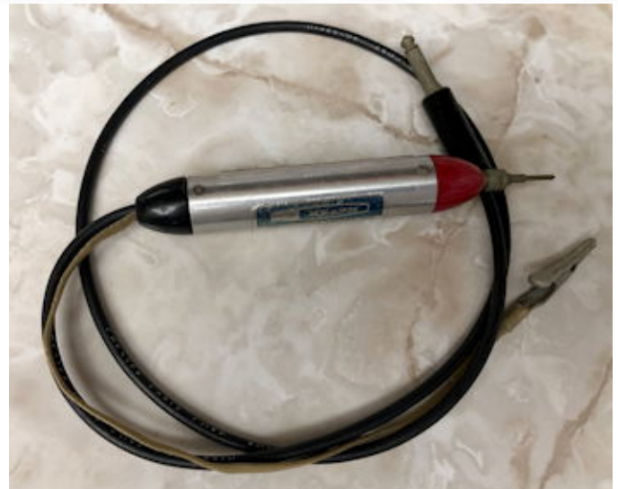
Figure 1: Heathkit #309-C RF Probe for all Heath VTVMs. Measures up to 30.V RF on up to 500 VDC (+ VRF).
