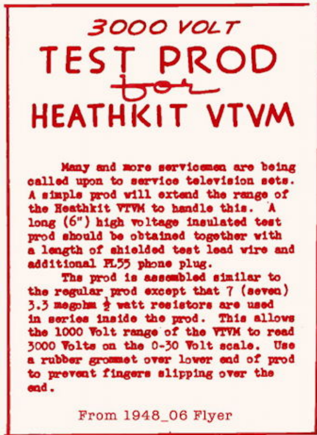
Figure 2: Tech note in the June 1948 Heath flyer discussing how to build a simple probe to extend the V-1 VTVM to measure 3 kV.
