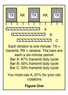
Exposure limits are also depend on the duty cycle of the mode you're operating. FM, SSTV, AFSK have a duty factor of 100%. SSB is between 20% and 40%. CW is 40% and a carrier is 100%. Again you can find the duty cycle for your mode in tables provided by the FCC and ARRL.
