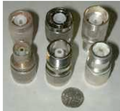
Top-(L to R) : Male C, HN and SC to 'Female N' Adapters Bottom-(L to R) : Female C, HN and SC to 'Male N' Adapters
