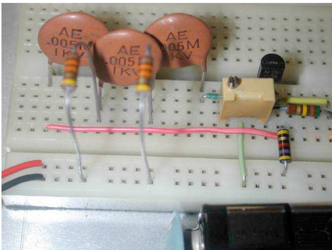
Figure 5: (Left) Is a photo of the phase-shift oscillator breadboard. Q1 is at the right immediately above the caramel colored trim pot (RE). The dark object to the lower right is a nine-volt battery.
