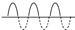
Figure 2b - Class B - The grid voltage reaches cutoff and plate current flows for 50% of a cycle.
