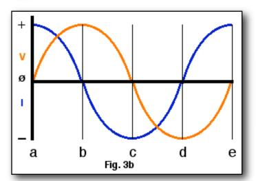
If the capacitor and inductor are perfect, so there is no energy loss, this oscillation will continue indefinitely as the energy moves between the coil and capacitor, swapping polarity each time.
