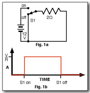
Inertia is a mechanical property that most are familiar with. If you push a car (on level ground) it's hard to get it moving, but once moving it tends to move easily and is hard to get it to stop. Inductance has a similar effect on current. The voltage created across an inductor is always in the direction that tends to resist the change in current.
