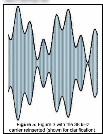
wave is at 90° (i.e. at its most positive point), and the black line in figure 4b is the locus of points when the phase of the 38 kHz carrier is at -90° (i.e. at its most negative point). [See Sidebar for more on degree notation]. Note that in figures 4a and 4 b the (L - R) subcarrier channel phase inverts with relation to the 38 KHz carrier each time the highlighted line crosses the X-axis.
