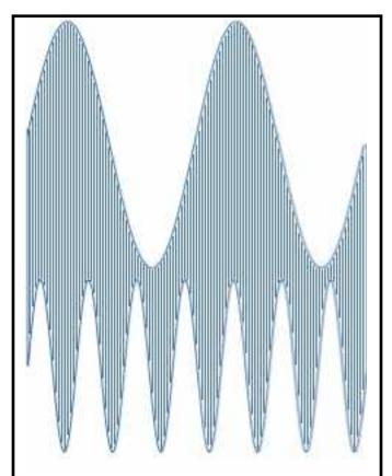
**Figure 7:** This is what figures 6 would all look like if the 38 kHz carrier was reinserted.
