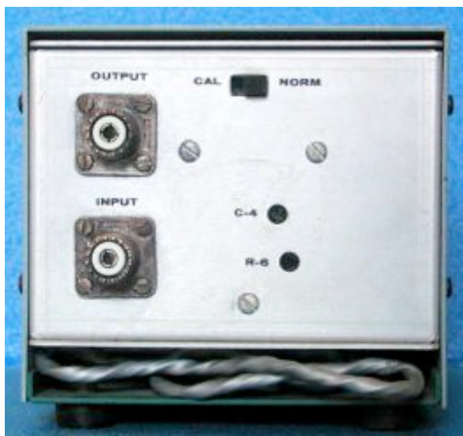
Fig 2: HM-102 Rear View. The sensor chassis may be removed for remote operation
