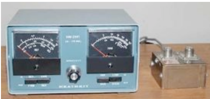
Figure 4 Heathkit HM-2141 Dual Meter VHF Wattmeter. The HM-2140 HF model is similar. The HM-2140A sports a brown motif to match the later Heathkit ham gear; otherwise it is unchanged.
