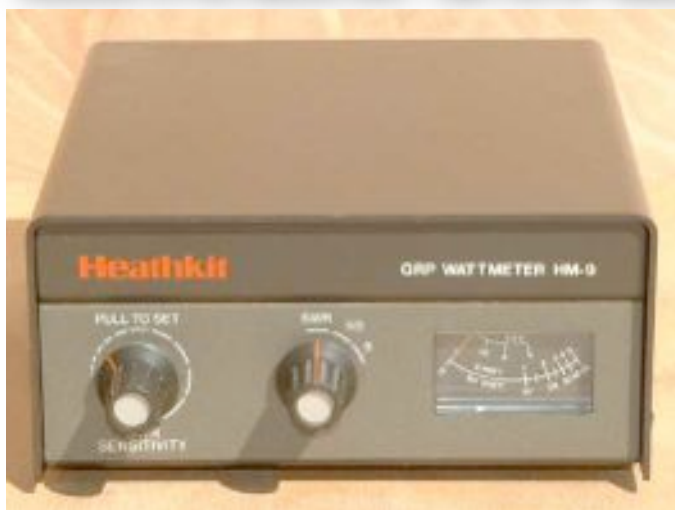
Fig. 5: Heathkit HM-9 QRP Wattmeter Be aware that the HM-9 could be wired for one of three bands: HF, 6-Mtrs or 2-Mtrs. Photo courtesy of - KC8RP
