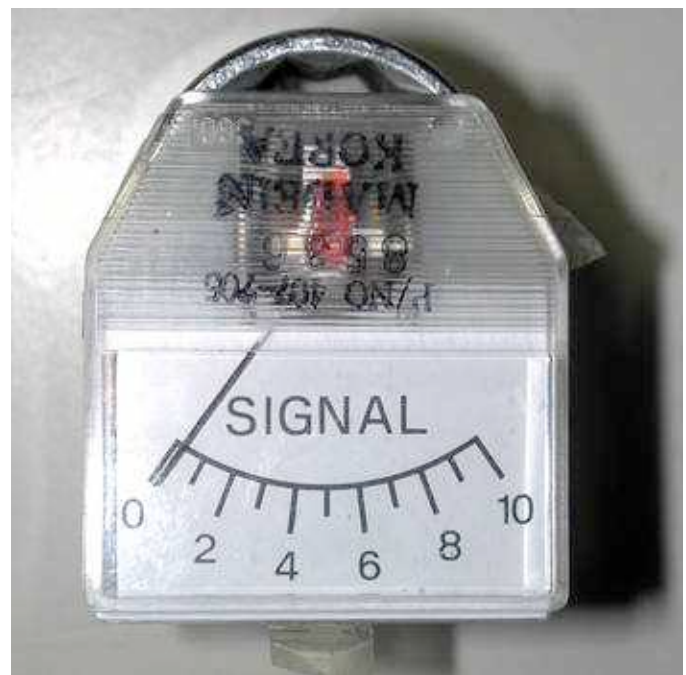
Figure 2: Sticking Meter from HD-1250
