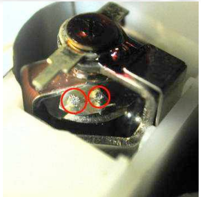
Figure 4: Circled are two glue type tail-weights. The side weights have already been removed from the coil top. Note the hairy growth on the left weight. This growth on a side weight caused the meter to stick.
