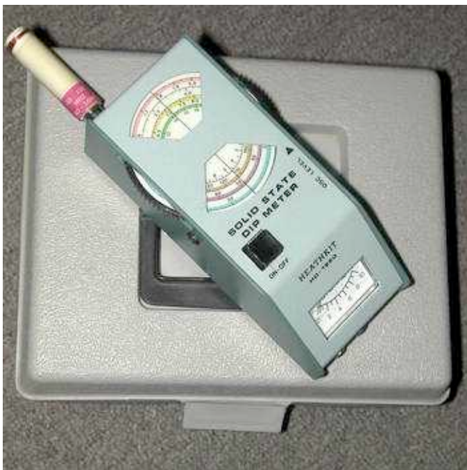
Figure 3: My Heathkit HD-1250 – Repaired, re-calibrated and sporting a replacement meter.
