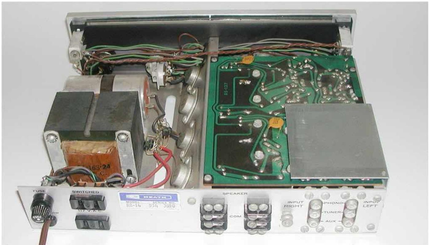
**Figure 5:** Rear view of the AA-14 Solid-State Stereo Amplifier showing rear connections, and circuit board. Power transformer is to the left and behind it the large 4,000  $\mu$ f main filter transformer, The four output transistors are on the sloping heat sink. *Photo courtesy of Don Peterson.*
