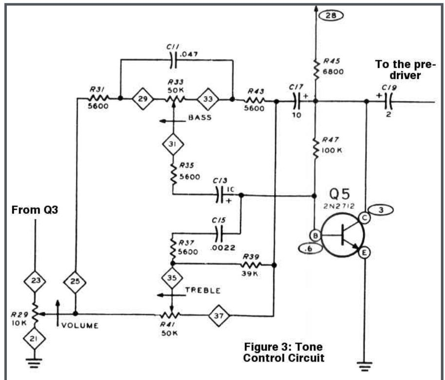
Figure 3: Tone Control Circuit
