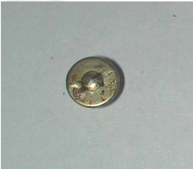
Figure 5: The silver disc contact prior to cleaning. The earlier switch contact was much dirtier to the point of being covered with black tarnish. However this had enough dirt to cause switch failure.
