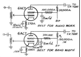
Figure 11: Gain modification suggestions from the June 1949 Heathkit Flyer.
