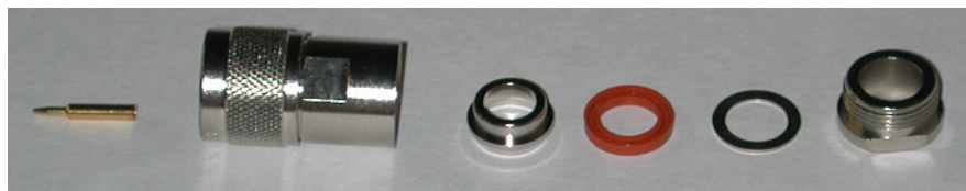
Parts of an “N” connector (Male shown) in assembly order. From left to right: Pin, Body, Clamp, Gasket, Washer, Nut.
