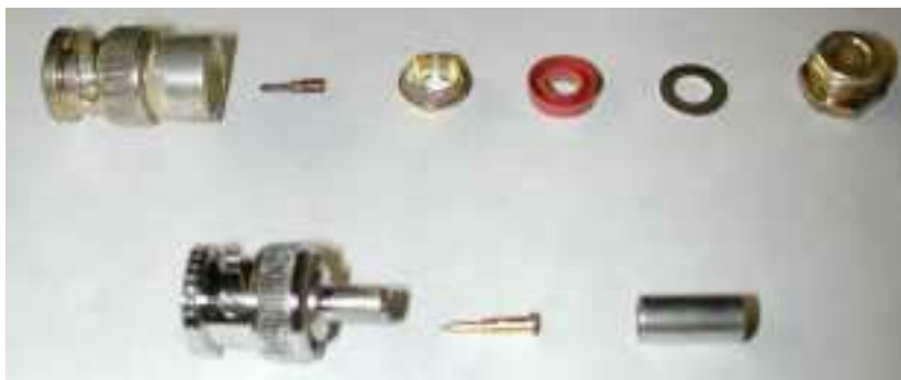
Top: UG-88C/U Clamp-Type BNC Connector in assembly order (Amphenol). Bottom: Pasternack PE4016 Crimp-type BNC Connector (Both fit RG-58/U)
