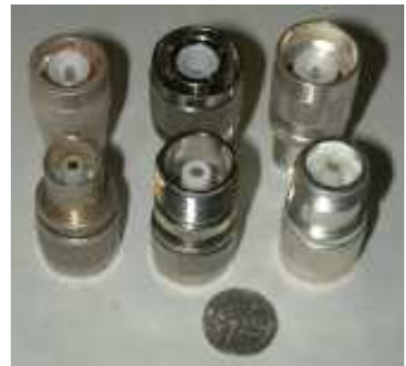
Top-(L to R) : Male C, HN and SC to 'Female N' Adapters
