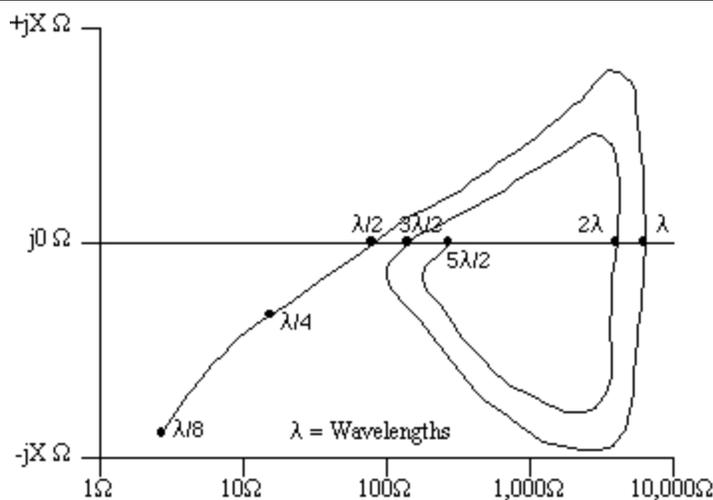
Figure 2: Antenna Feedpoint Impedance vs. Antenna Length
