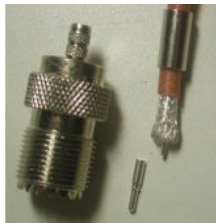
Figure 2 - Photo of prepared end of RG-142/U coax with trim dimensions for female UHF crimp connector (Wireman #1147)
