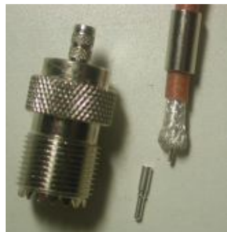
Figure 2 - Photo of prepared end of RG-142/U coax with trim dimensions for female UHF crimp connector (Wireman #1147)
