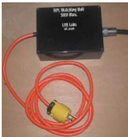
Figure 2 - The prototype RPL matching unit. Though marked for 5 KW, this unit really only handles 3 KW. Note the 25A AC plug.
