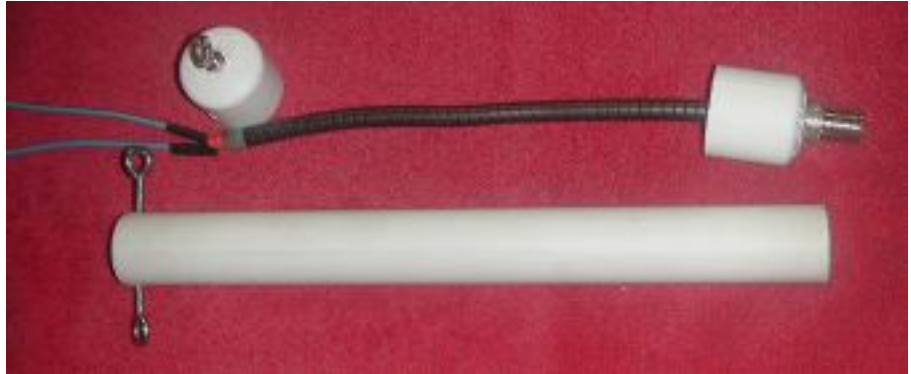
Figure 4 - The balun, with enclosure, ready for final assembly.
