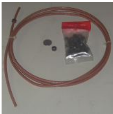
Figure 1 - RG-142/U and bag of 50 FB-73-2401 ferrite beads. Dime is included for size comparison.
