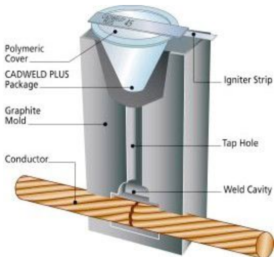
Figure 1 – Cross section of a typical exothermic welding mold. (Courtesy of ERICO CADWELD® PLUS)
