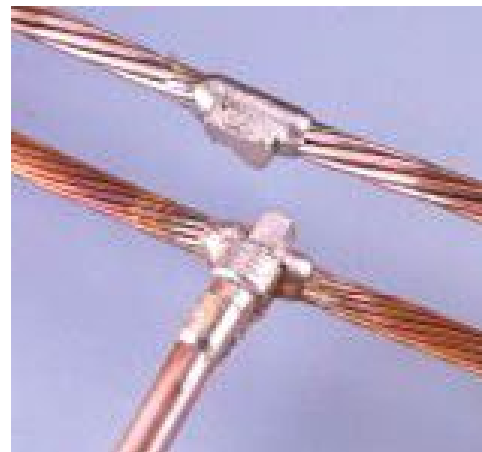
Figure 2 – The resulting welded wires. (Courtesy of ERICO CADWELD® PLUS)
