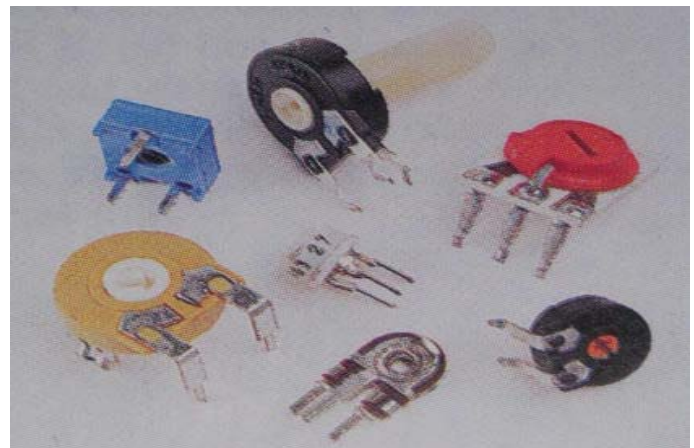
Figure 6 – Small potentiometers and trimmers often used for variable controls in electronic circuits.
