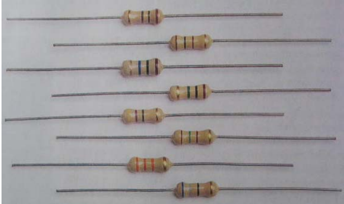
Figure 1 – Typical carbon-composite resistors.
