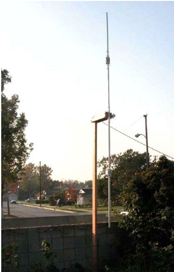
Figure 1 – 30M Shortened Dipole Mounted as a Vertical on Simple Tower
