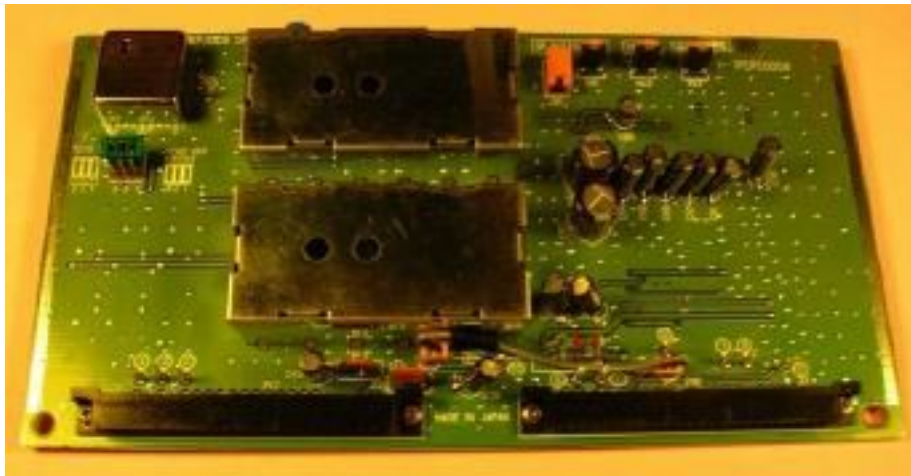
REF/DSS Card with TCXO Installed
