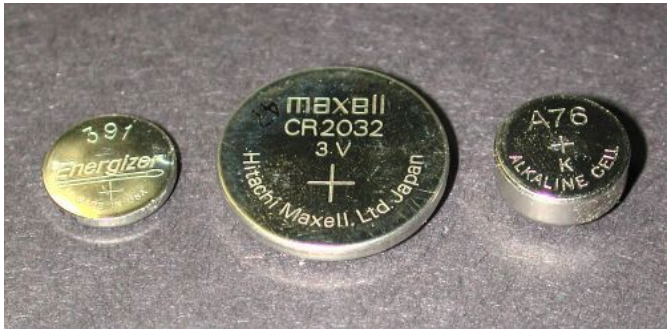
L to R - SR 1120W (391) Silver Oxide, CR2032 Lithium and LR1154 (A76) Alkaline Coin Cells
