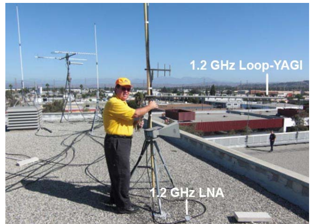
Figure 3 – Robbie KB6CJZ Adjusts RCVR Loop-Yagi
