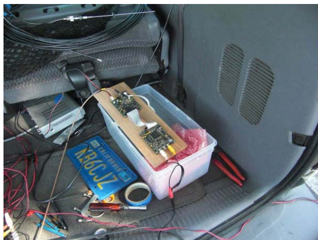
Figure 1 – DATV DVB-S 1 mW Transmitter for 1.2 GHz
