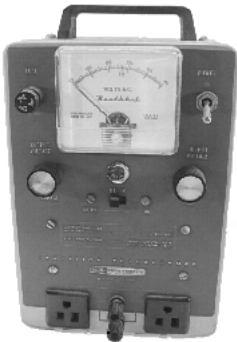
Later Heathkit IP-22 Isolation transformer
