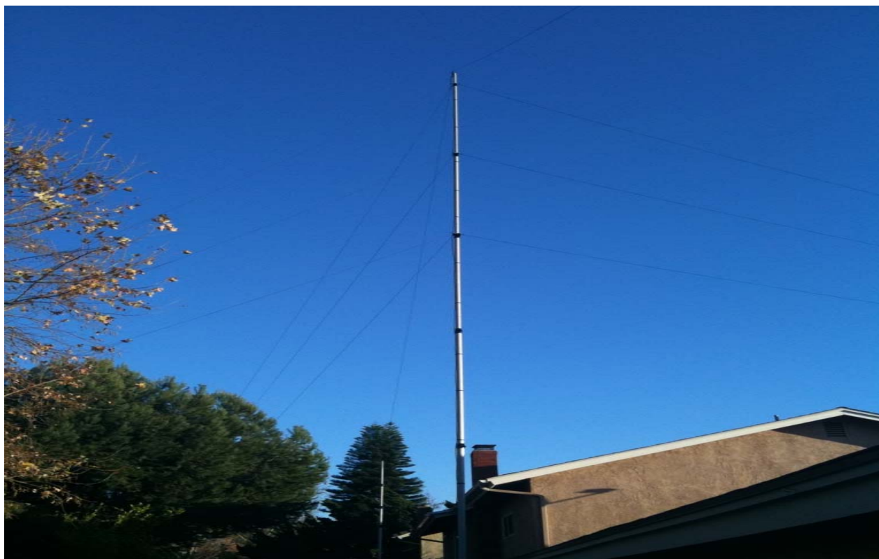
A view of the HF dipole from the backyard; fiberglass masts made by Max Gain Systems
