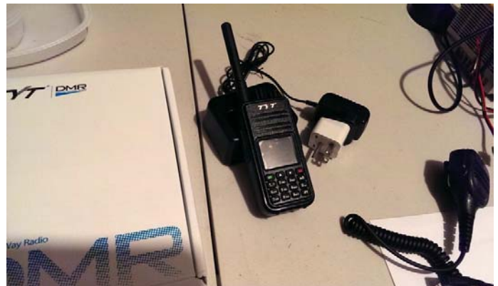
The TYT MD-380 UHF radio operates 400-480 MHz
