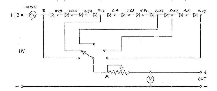
Optional features are selector switch, trimming potentiometer and meter. The pot should be 50 ohm or less impedance and 5 or more watt. If 1 amp or less is sufficient, Radio Shack sells a pack of 40 diodes for about \$2.00. Select a fuse to suit the components used.
