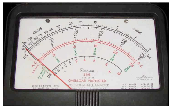
Figure 4: Simpson 260-7F VOM Meter Scale
