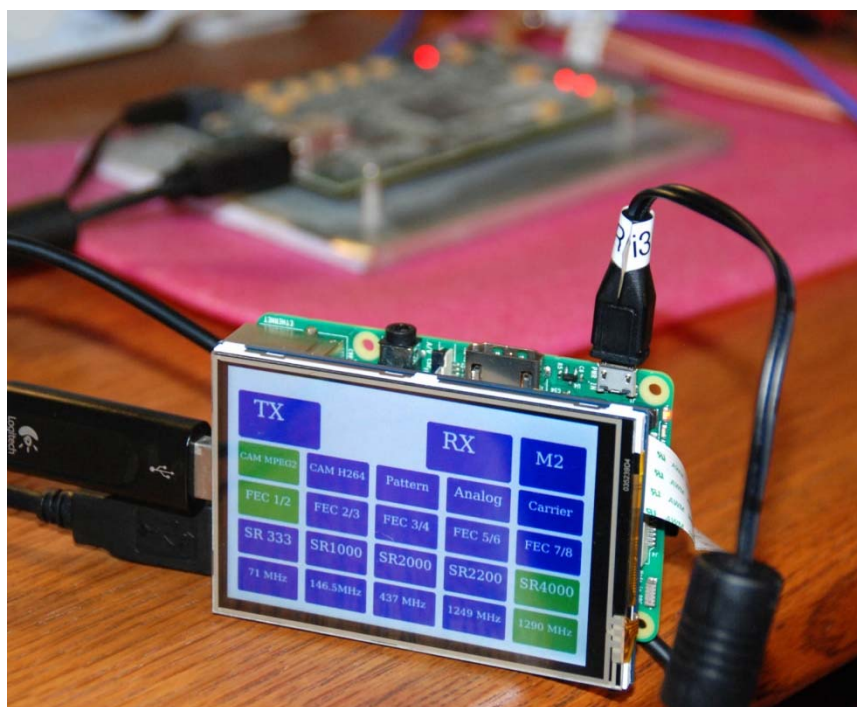
Portsdown Project using RPi-3 / RpiDATV SW / DATV-Express modulator
