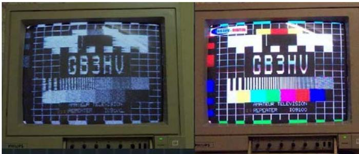
**Fig 3 – Comparison of analog PIX and DATV PIX using the same antennas with weak sigs**
