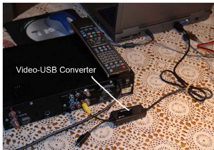
Figure 6 – The Composite-Video-to-USB converter Sends the Video to the Computer USB Port
