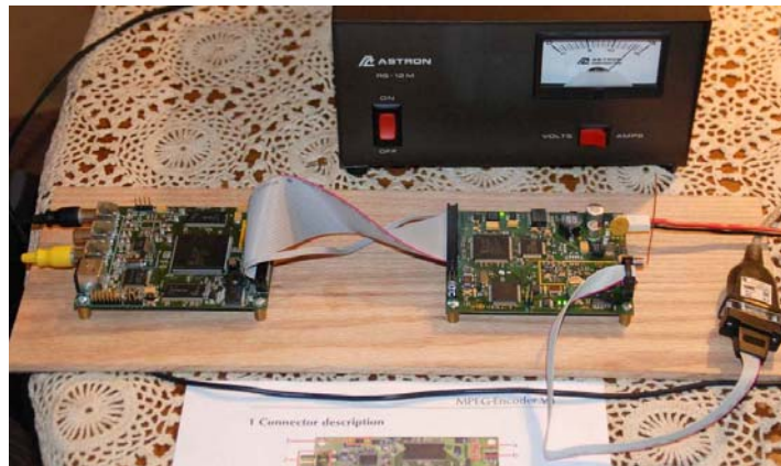
Figure 1 – MPEG2 and DVB-S 1.2 GHz Exciter Boards from SR-Systems on the Test “Breadboard”
