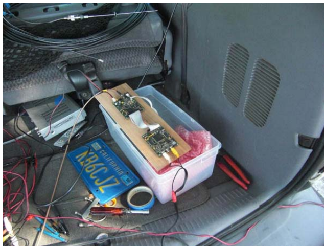
Figure 1 – DATV DVB-S 1 mW Transmitter for 1.2 GHz
