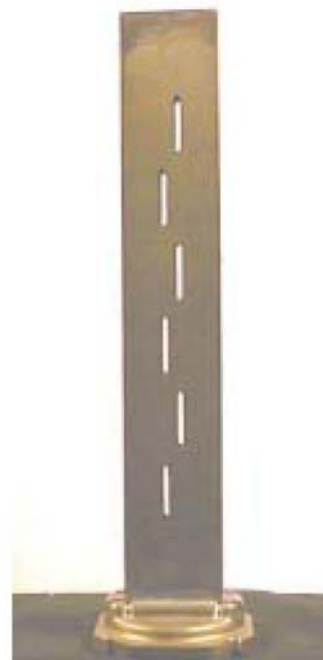
Figure 2 – 10 GHz Slot Antenna made from WR-90 Waveguide with 12-slot array (Courtesy of Paul Wade W1GHZ.org)
