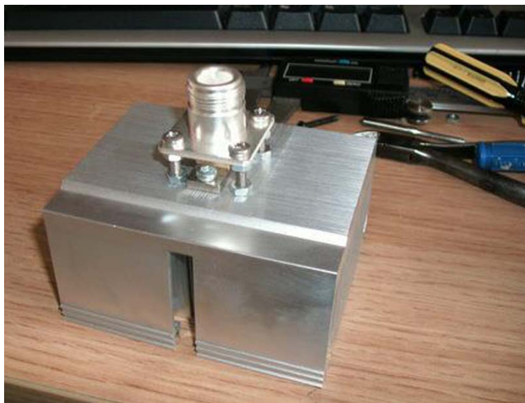
Fig 1 – Completed Dummy Load with flange-resistor and N-connector installed on Heat Sink, but no fan.
