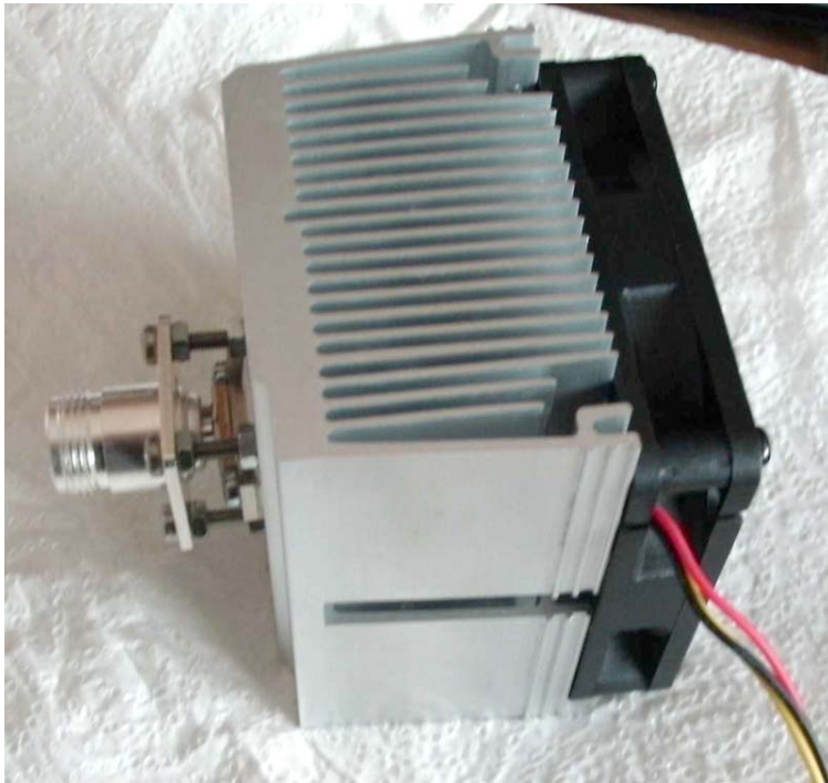
Fig 3 – Completed Dummy Load unit now fitted with a 12V cooling fan
