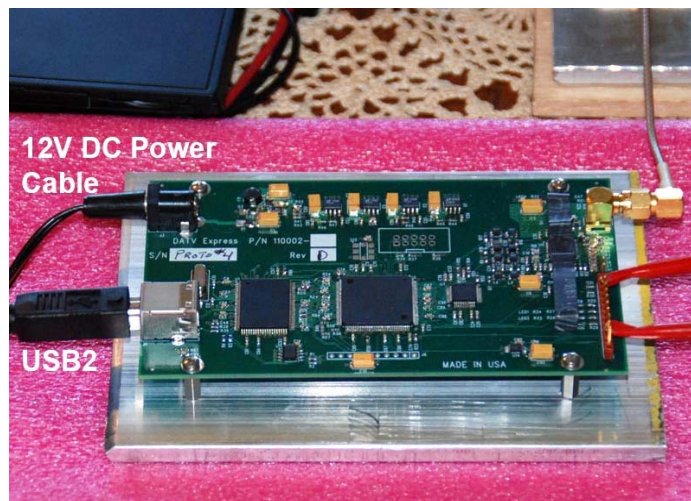
Figure 2 – The DATV-Express exciter hardware board is fitted with an aluminum plate as a heat-spreader
