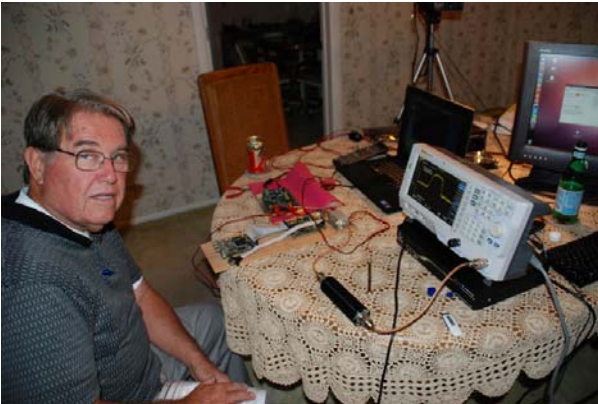
Figure 06 – KB6CJZ is shown after connecting an external 20 dB attenuator from Kuhne RF amp
