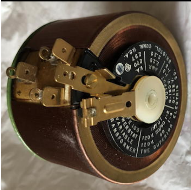
Figure 4: A variable autotransformer similar to T1 that is used in the IP-5220. This is a Powerstat 10B made by the Superior Electric Company.
