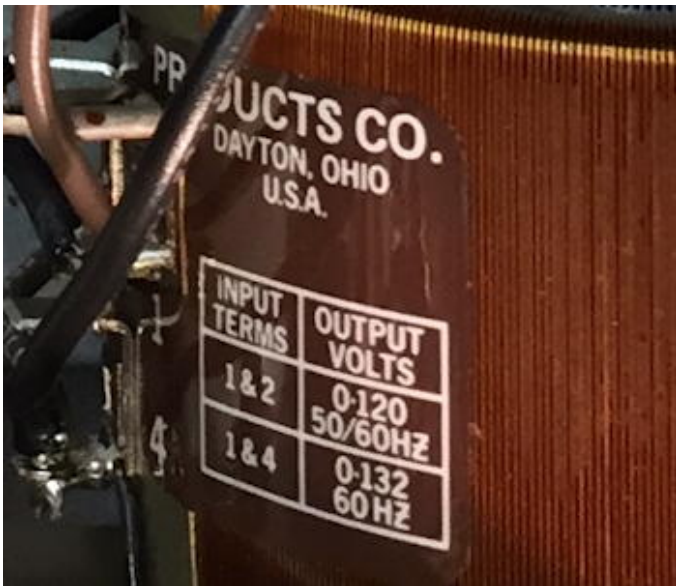
Figure 7: T1 is believed to be made by Staco Power Products of Dayton, Ohio. Note when the input terminals 1 & 4 are used, the output is 132 V, not 140 V. Also note that using terminals 1 & 4 the transformer may not be used at 50 Hz.
