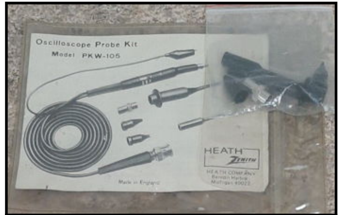
Figure 14: Heath PKW-105 factory wired probe instruction book and accessories.
