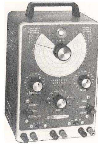
So what does the IT-11 do? It measures capacitance from 10 pF to 1000  $\mu$ F. and it checks capacitors for leakage at DC test voltages from 3 to 600 volts. The IT-11 also measures the power factor of electrolytic capacitors. But the IT-11 does even more. It measures resistors from 5  $\Omega$  to 50 M $\Omega$ ; and with a small supply of known inductors it will measure unknown inductances. You can also measure the turns ratio of power and audio transformers.
