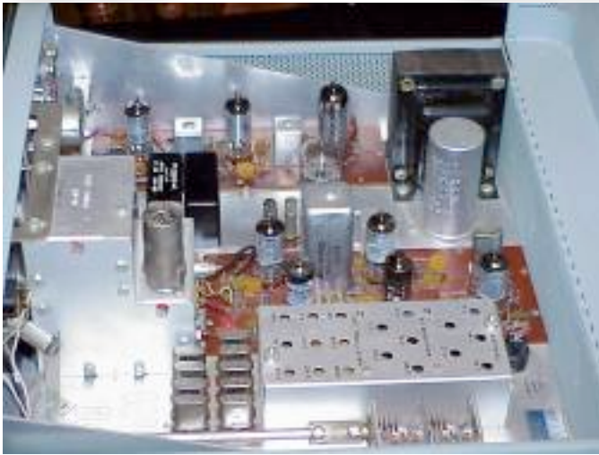
Figure 3: Heathkit SB-301 interior view.
