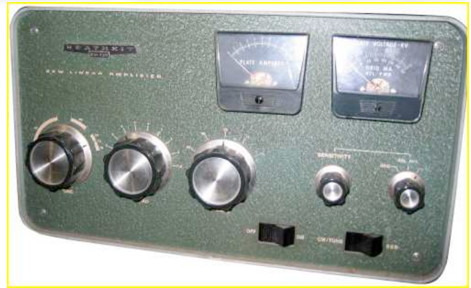
Fig. 1 SB-220 2KW Amplifier. The SB-221 looks identical except for the 10 meter band switch markings.
