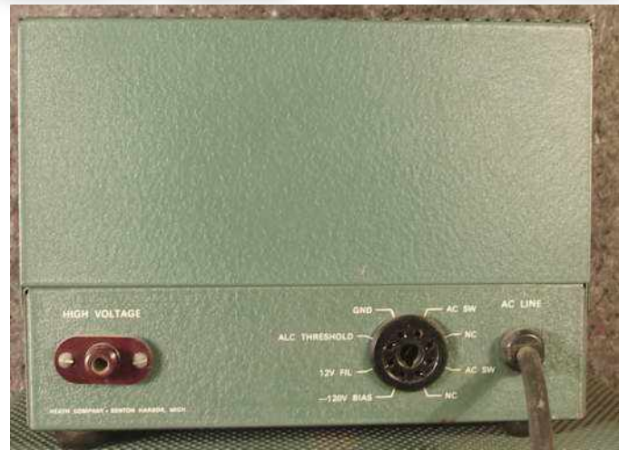
Figure 6: HP-24 AC Power Supply Photo courtesy of Dave Lien -W6OVP
