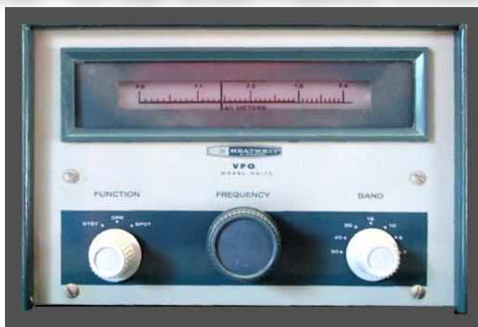
Figure 1: Heathkit HG-10 VFO
